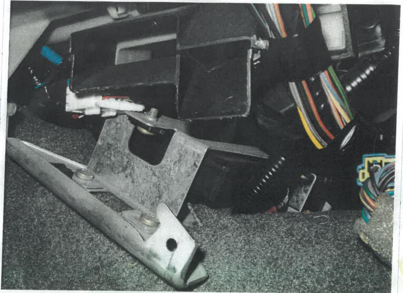
On removing the passenger's side panel, you will see a metal cage held by two torx bolts; within it, a black plastic box; this is the immobiliser. You will have greater access to these bolts if you remove the black plastic heater vent by unclipping it.
